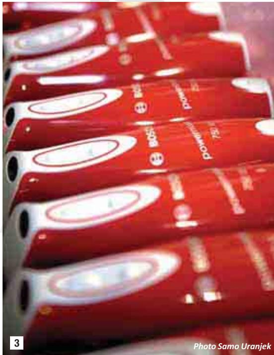
**3** Plasma treatment by means of the patented rotation jet RD 1004 imparts a perfect appearance also to dark, high-gloss polypropylene and ensures strong adhesion of the printing paint.
