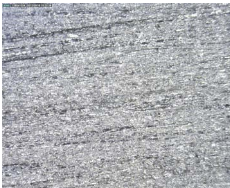
Fig. 4: Micro-cavities in the three-dimensional honeycomb structure have collapsed: At this stage it is no longer possible to apply wax. (Photo: Scuola Skiman)
