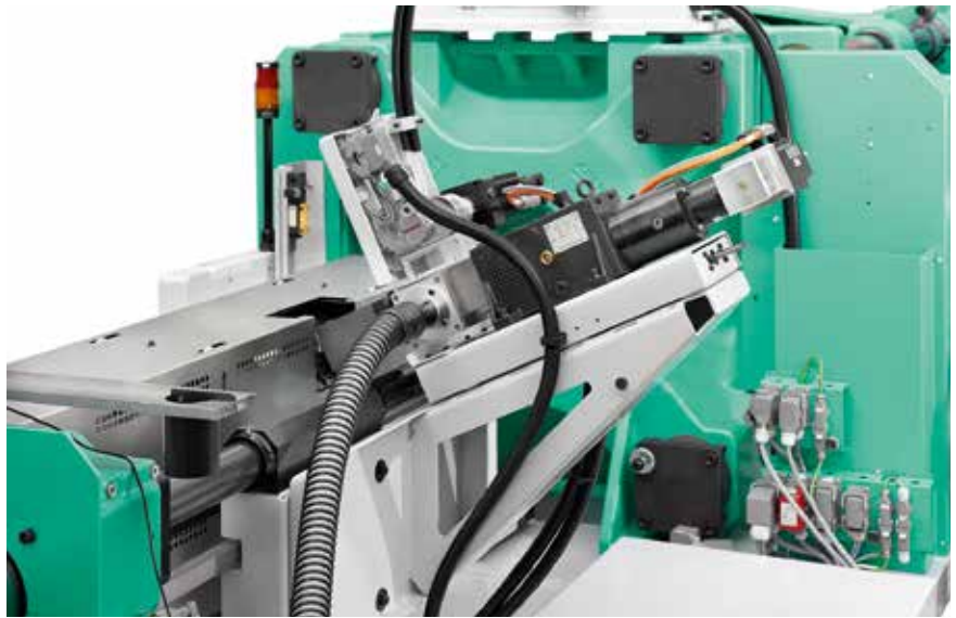
Fig. 3. Section of the FDC unit with fiber cutting and feed at the front part of the injection unit (© Arburg)
