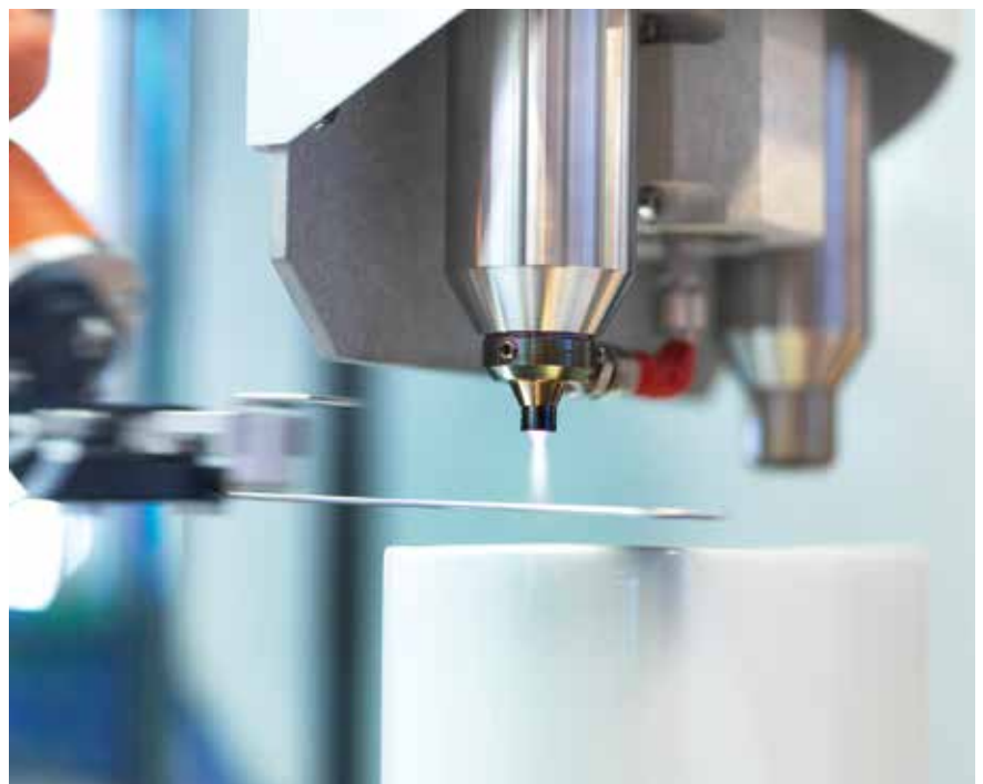
Fig. 6. Application of a plasma polymer layer to sheet metal by the "Plasma-SealTight" nozzle
