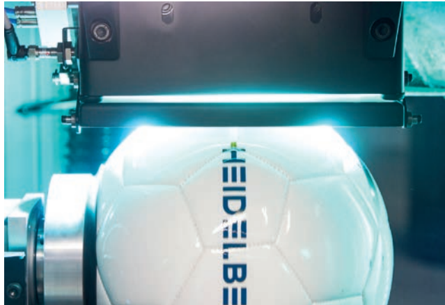
Fig. 2. Four-color UV inkjet digital printing: The energy-saving UV LED system ensures that inks in the Omnifire cure in a matter of seconds (© Heidelberg Druckmaschinen)
