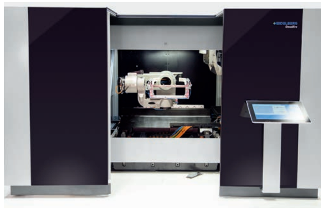
Fig. 4. Six-axis robotics: The Omnifire 1000 can print free-form objects of any shape up to 1.4 m long, from ice hockey sticks to suitcases (© Heidelberg Druckmaschinen)
