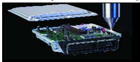
Pretreatment and activation of the housing before adhesive application.
