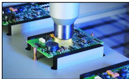
Openair plasma provides microfine cleaning and surface preparation which ensures long-term adhesion of encapsulating hotmelt.
