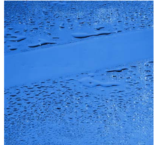
Pretreatment with Openair®-Plasma causes a holohedral wettability of material surfaces. The straight line shows the plasma treated part of the substrate. (Foto: Plasmatreat)
