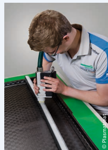
Fig. 10: Openair plasma treatment of the rigid foam rib using a hand-held rotary nozzle.
