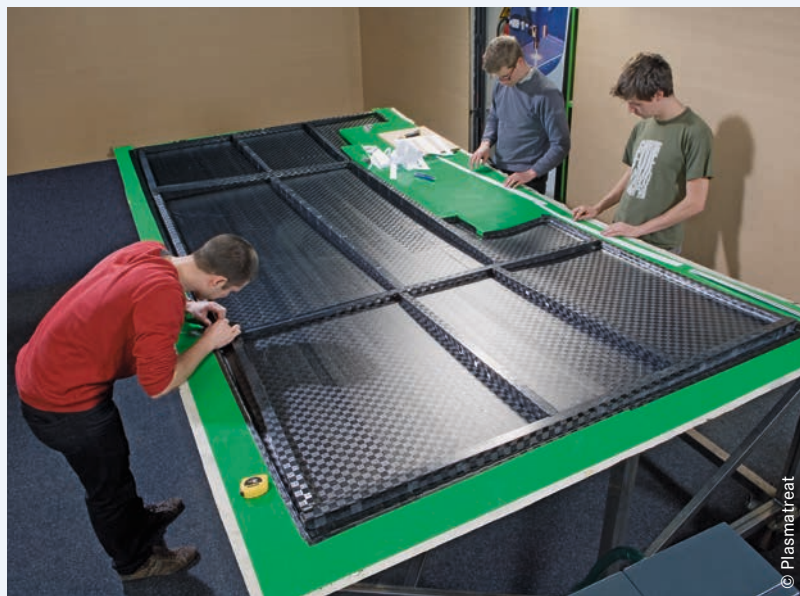
Fig. 12: The monocoque outer shell receives its final stiffening rib.
