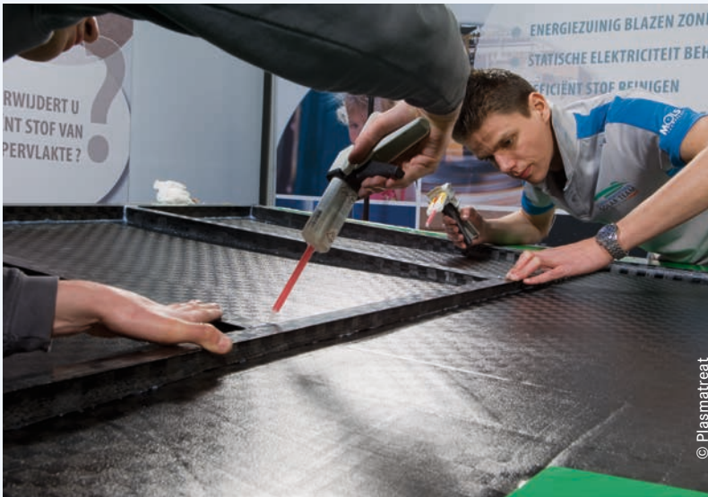
Fig. 11: Immediately after plasma treatment, the rib is bonded with a 2-component epoxy adhesive.
