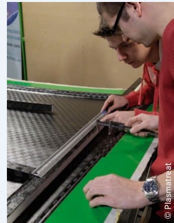
Fig. 9: Production manager Dokus Soetemans measures and marks the adhesive surface with millimeter precision.
