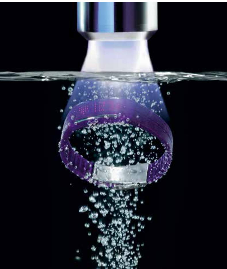
Water-tight: The atmospheric pressure plasma nozzle technology developed by Plasmatreat around 20 years ago can now be used to produce corrosion-resistant bonds for hybrid components (© Plasmatreat)
