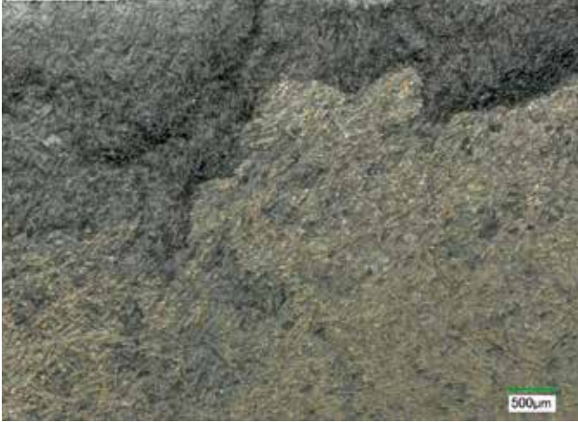
Fig. 3. Mixed fracture under the microscope: Some of the glass fibers from the polyamide compound are firmly anchored in the plasma polymer layer (© Akro-Plastic)
