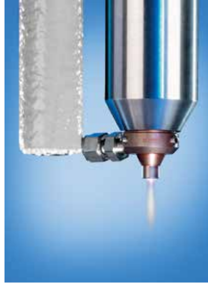
Fig. 2. Atmospheric PlasmaPlus technology: The chemical-physical coating process enables the area-selective application of functional nanocoatings and the formation of covalent bonds between different materials
