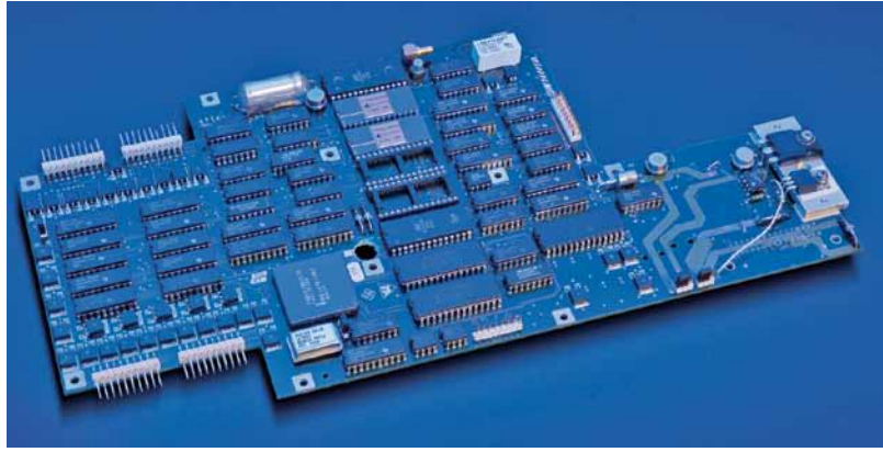
Fig. 5. The coating's adhesive bond is visually inspected under UV light before the SMD assembly is mounted in the radio. Then a Burn-In test is performed to verify its stability (Photo: Plasmatreat)
