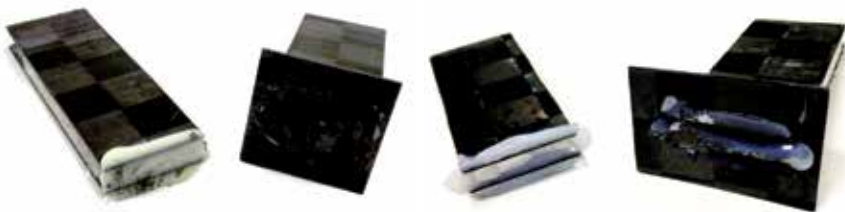
Adhesive fracture before plasma treatment (left) and cohesive fracture after plasma treatment (right)
